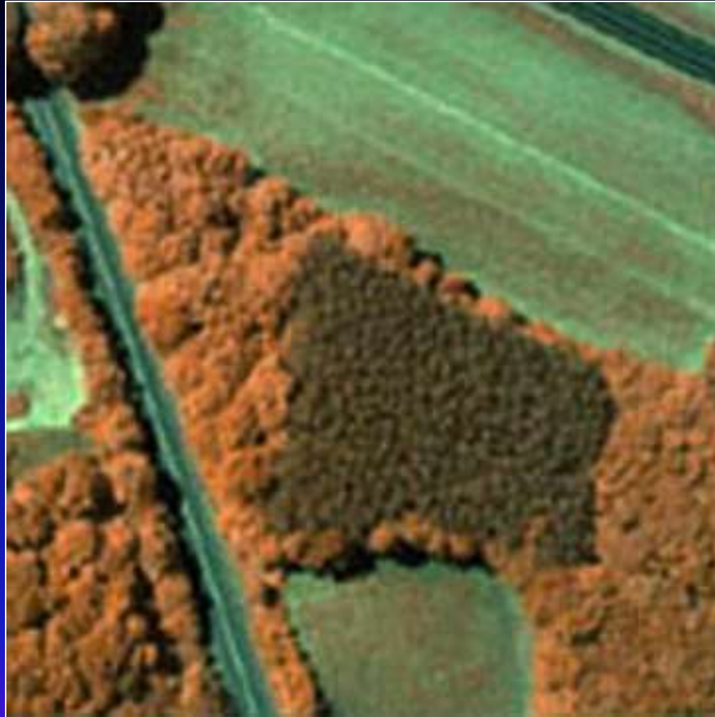
Deciduous versus coniferous forest at 1 x 1 m recorded by Spatial Emerge digital camera in green, red, and near-infrared bands
