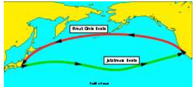
Flights between Tokyo and Los Angeles using the jet stream eastbound and a great circle route westbound.
