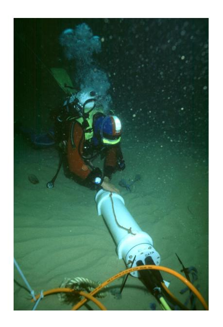
Wave recorder on the seabed (with steel subframe buried in the sand), connected to an array of six pressure transducers. The system was used to measure incident and reflected waves.
